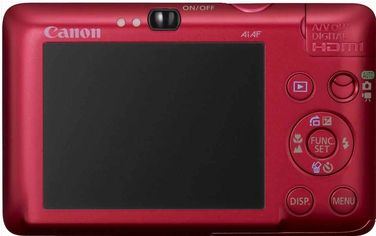
This image shows the rear of the Canon PowerShot SD780IS camera. Prominently featured is the 2.5-inch PureColor LCD II screen. To the right of the screen are the control buttons, including the directional pad with FUNC./SET button, playback button, menu button, and display button, along with the power switch at the top.
