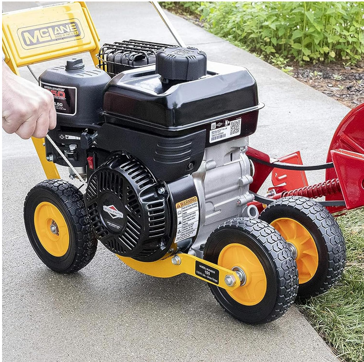
Figure 3: Engine close-up, showing the fuel tank and oil fill locations.
