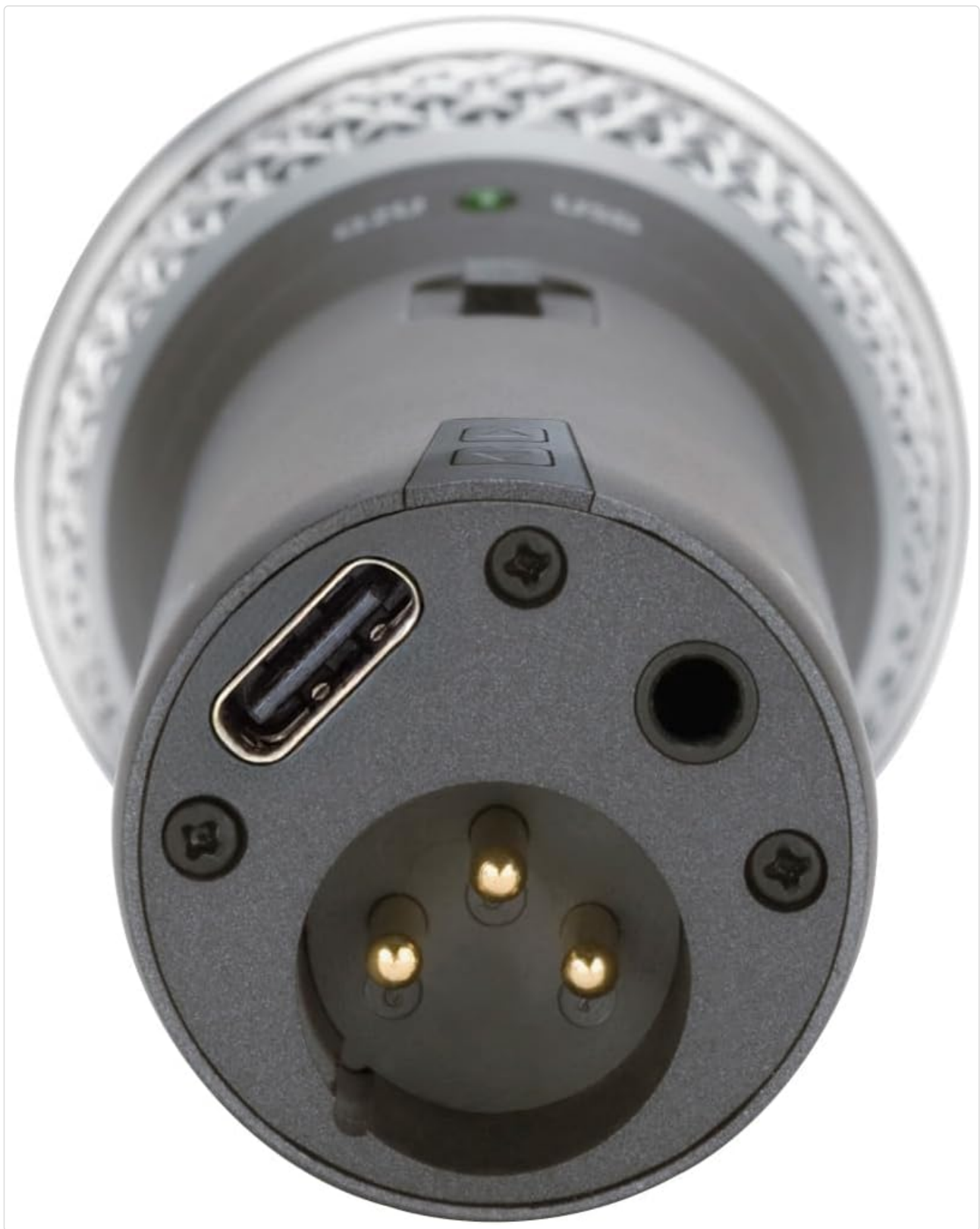
Image: Bottom view of the SAMSON Q2U microphone, highlighting the XLR, USB-C, and 3.5mm headphone jacks.
