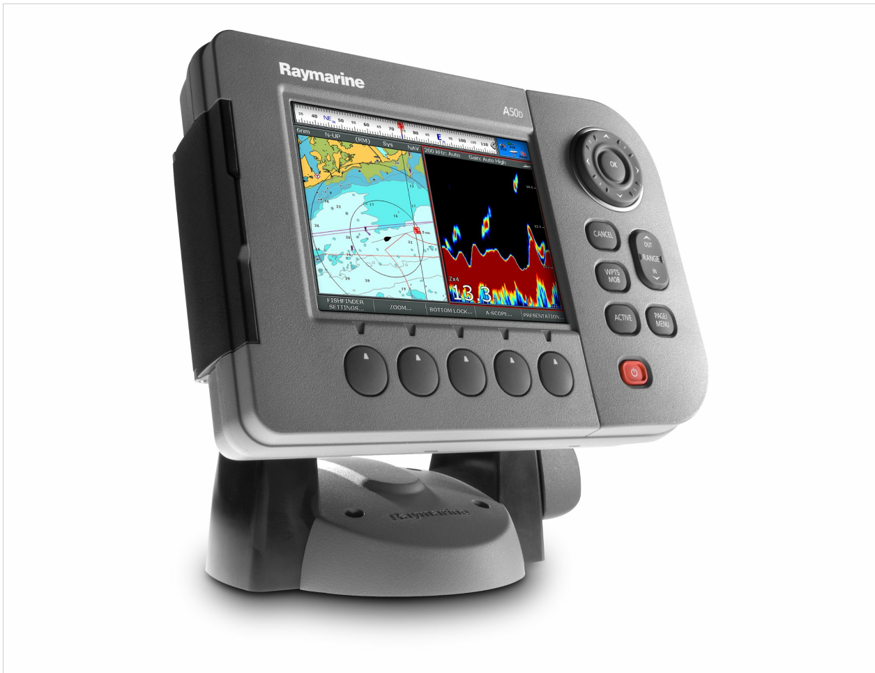
Figure 1: Raymarine A50D unit showing the display, control buttons, and mounting bracket. The screen displays both chartplotter and fishfinder data simultaneously. Key controls include a directional pad with an 'OK' button, 'CANCEL', 'OUT/IN RANGE', 'WPTS/MOB', 'ACTIVE', 'PAGE/MENU', and dedicated soft keys below the screen for 'FISHFINDER SETTINGS', 'ZOOM', 'BOTTOM LOCK', 'A-SCOPE', and 'PRESENTATION'. A red power button is located at the bottom right.
