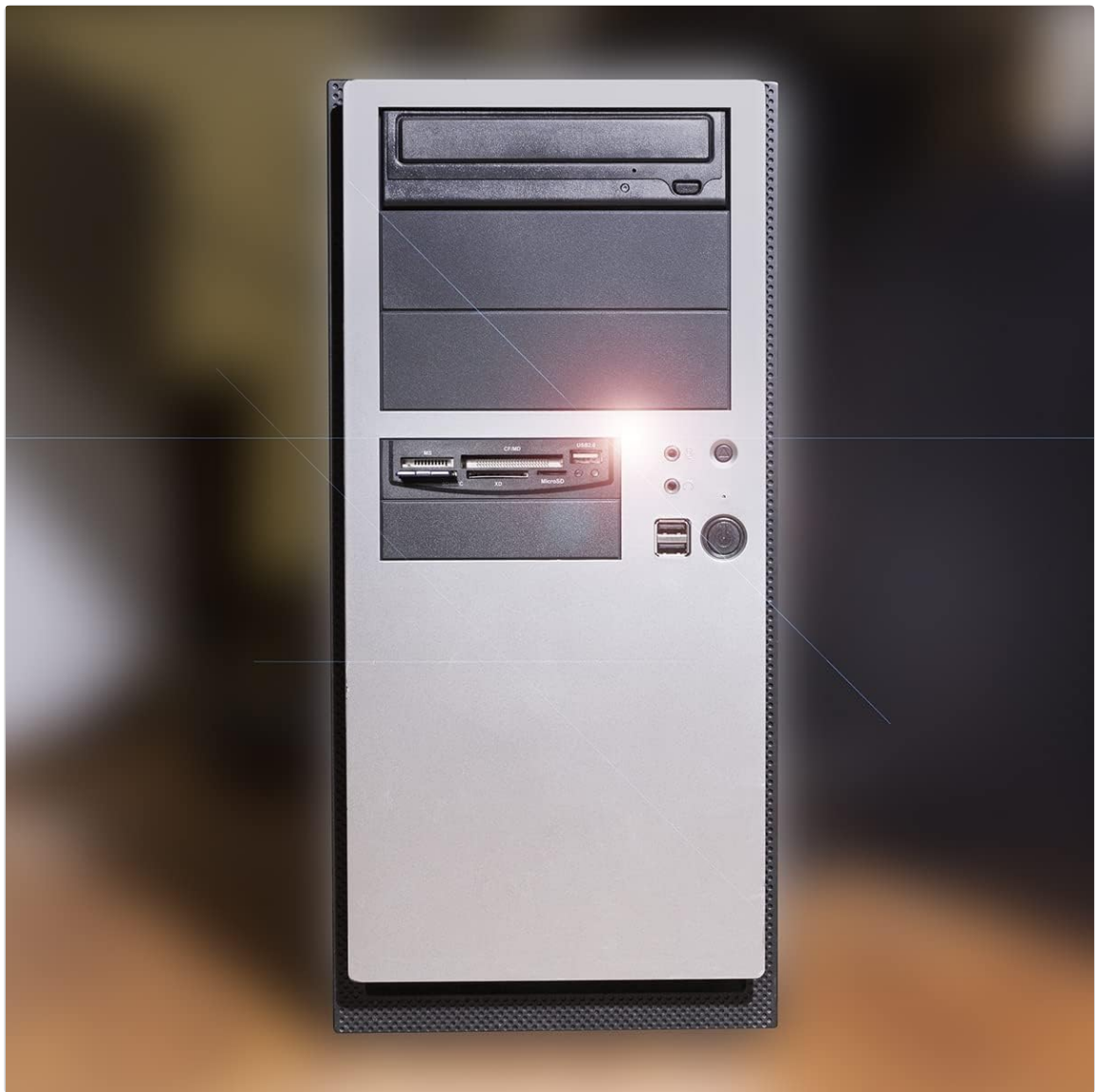
Image 3.1: The LogiLink CR0012 Multi-Card Reader shown installed in a desktop computer's 3.5-inch drive bay, integrated into the front panel.
