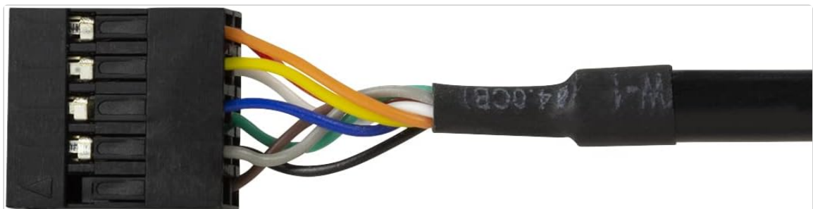
Image 3.2: Close-up view of the internal 9-pin USB 2.0 header cable, which connects the card reader to the computer's motherboard.
