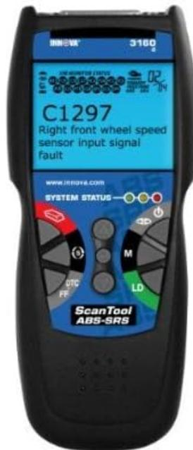
*Image: The Innova 3160 screen showing a C1297 ABS code, indicating a right front wheel speed sensor input signal fault.*
