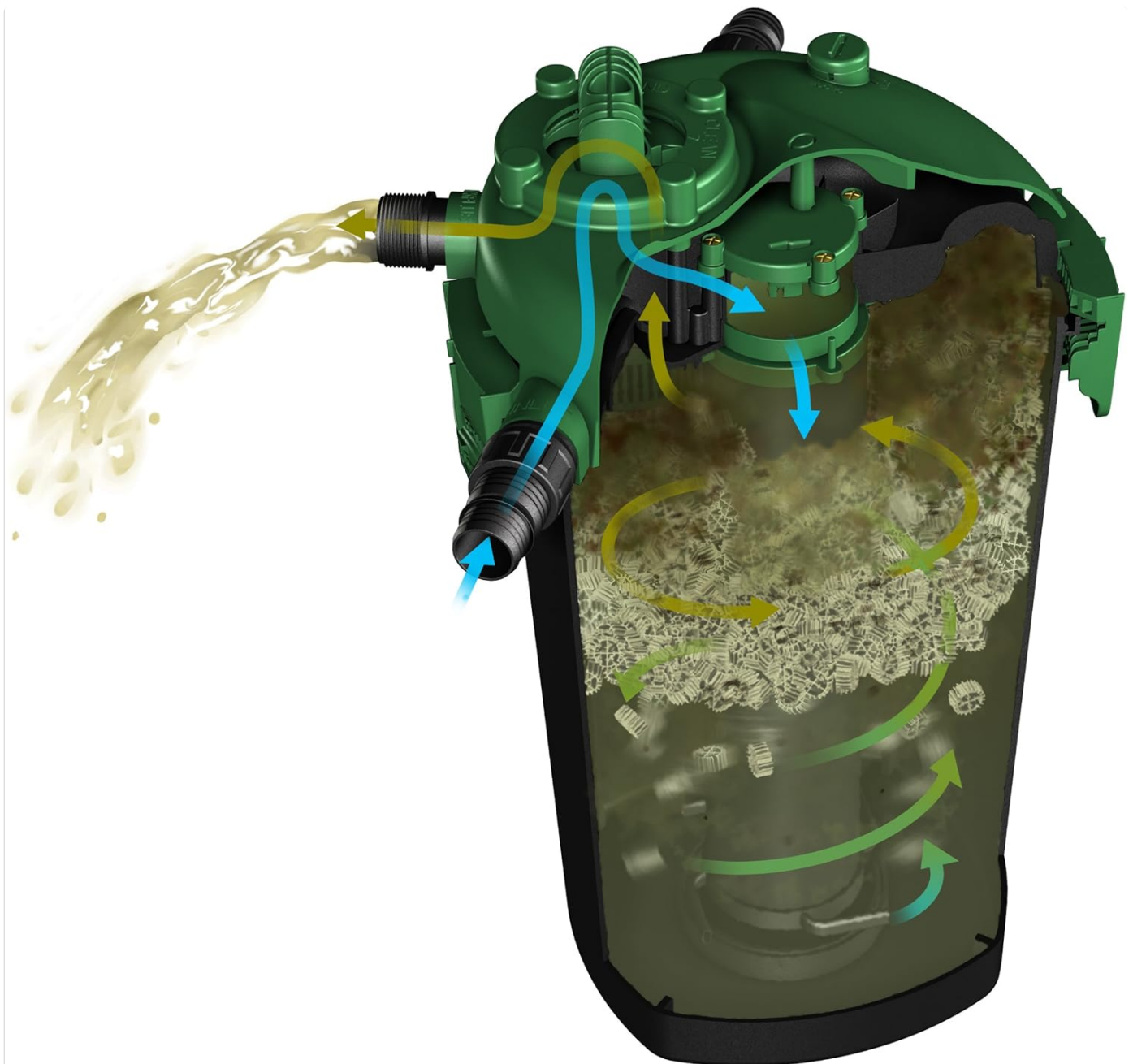
Figure 2: Illustration of water flow and mechanical filtration within the filter, showing debris being trapped.
