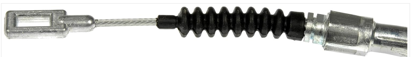
Image 5.1: Close-up of one end of the Dorman C660047 cable, showing the attachment mechanism. This end typically connects to the parking brake lever or an equalizer.
