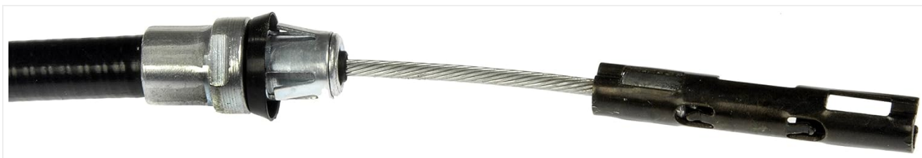
Image 5.2: Close-up of the other end of the Dorman C660047 cable, showing the cable housing and connection point. This end typically connects to the rear brake assembly.
