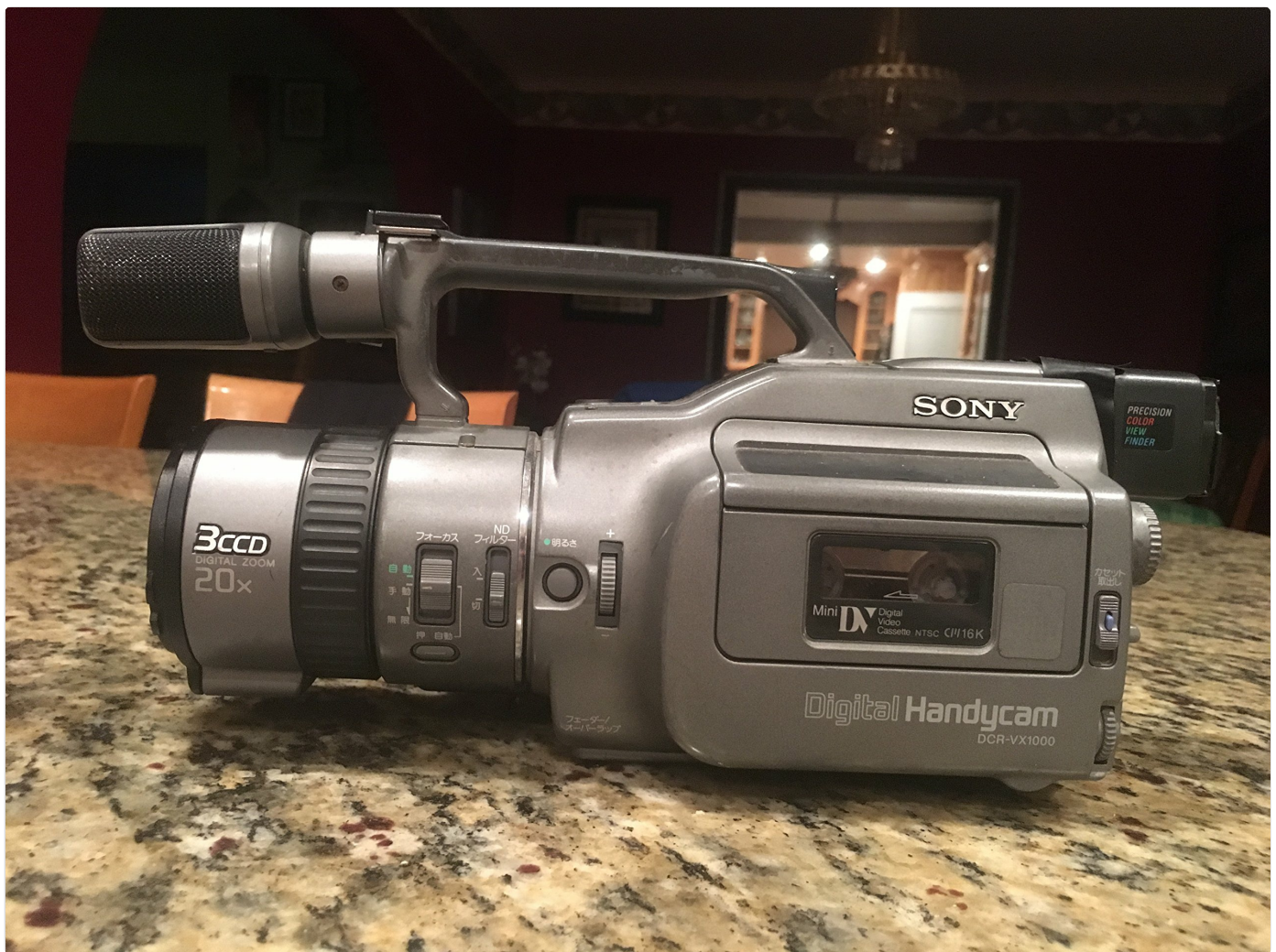
Figure 1: Left side view of the Sony DCR-VX1000 Digital Handycam. This view highlights the lens with its 3CCD and 20x digital zoom markings, along with manual controls for ND filter, focus, and brightness. The Mini DV tape compartment is also visible, labeled "Digital Handycam DCR-VX1000".
