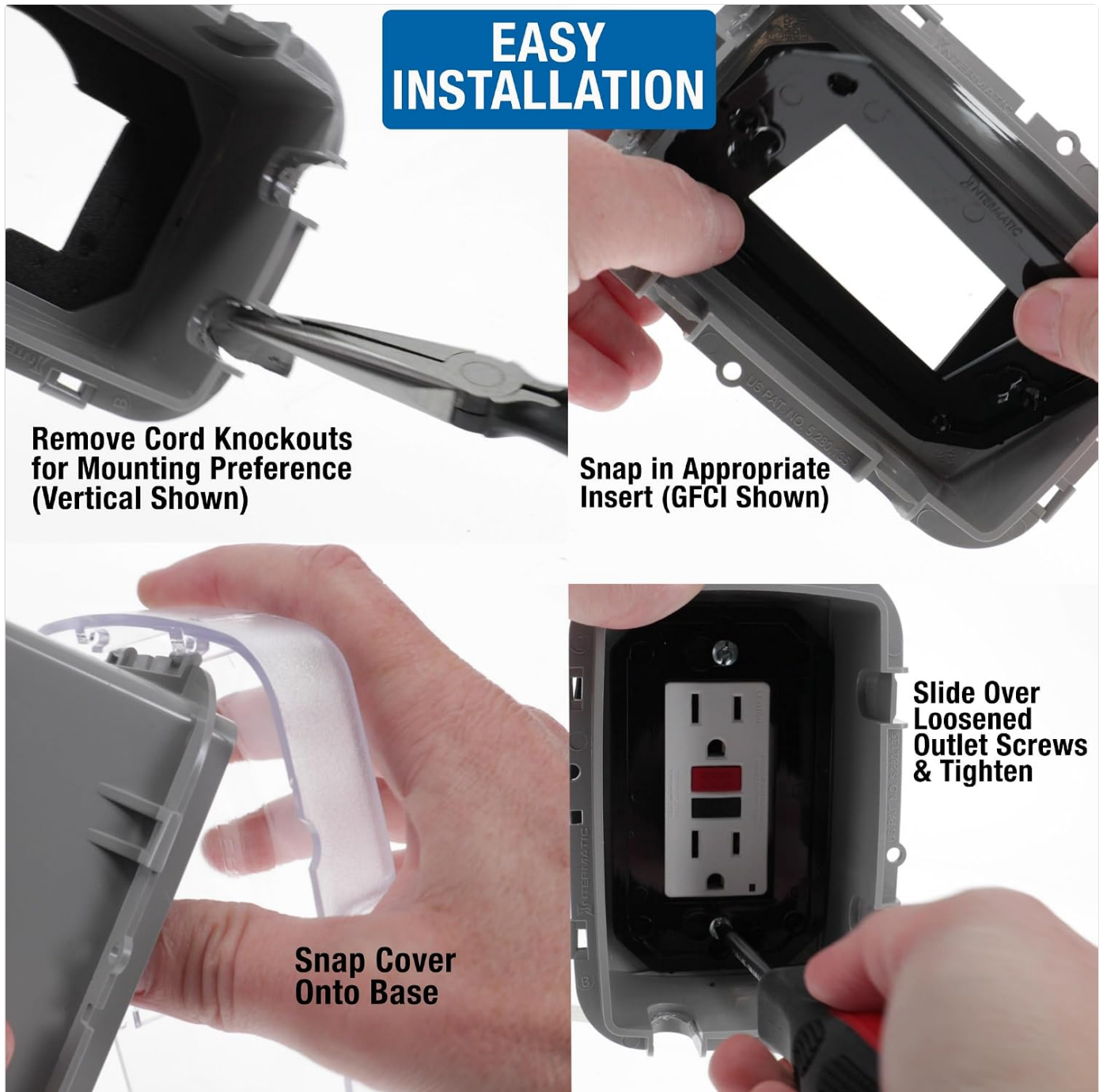
Figure 3: Step-by-step installation process for the WP3100C.
