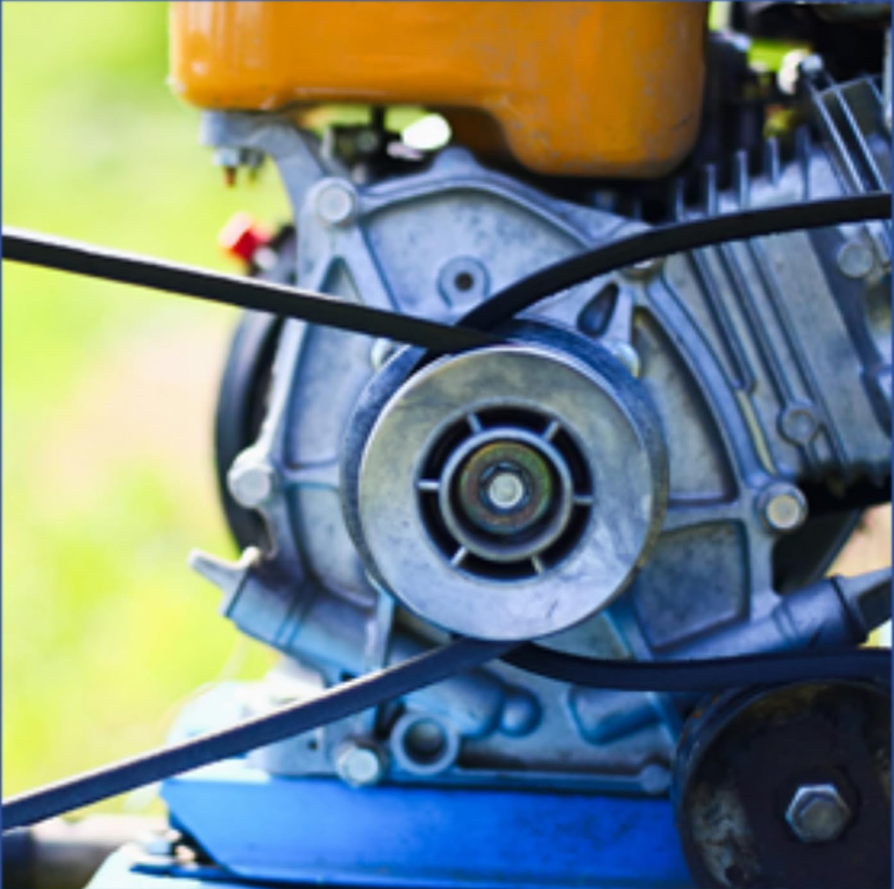
Image 4: A close-up view of a belt properly installed on an engine's pulley system, demonstrating correct routing.
