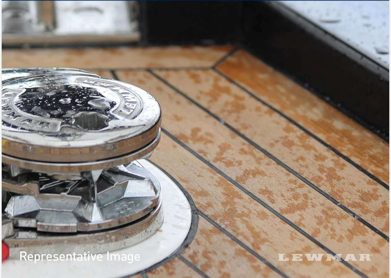
Figure 2.2: The windlass is constructed from tough stainless steel for durability and protection.
