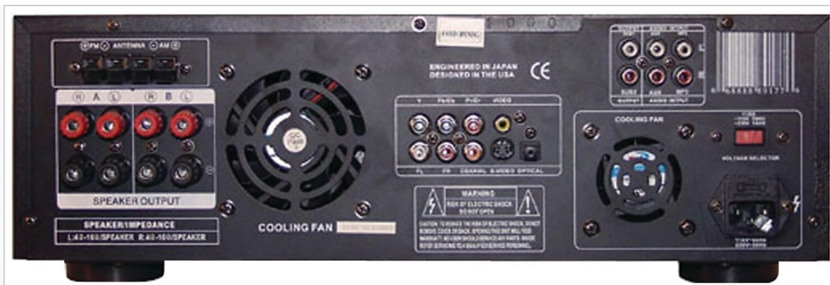
Image: Rear view of the Pyle PD1000A receiver, detailing speaker output terminals (A and B), RCA audio/video inputs and outputs, AM/FM antenna connections, and the power input with voltage selector.
