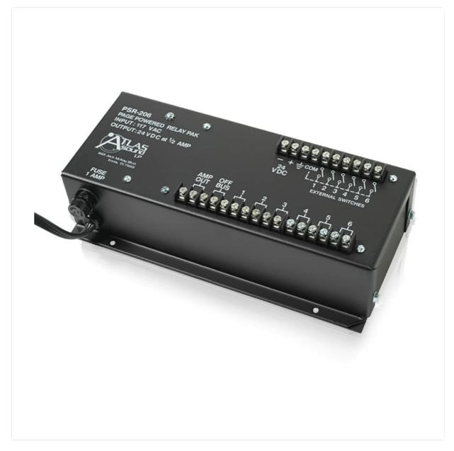
Figure 1: Top view of the AtlasIED PSR-206 showing power input, fuse, amplifier output, bus connections, 24 VDC output, and six external switch relay terminals.
