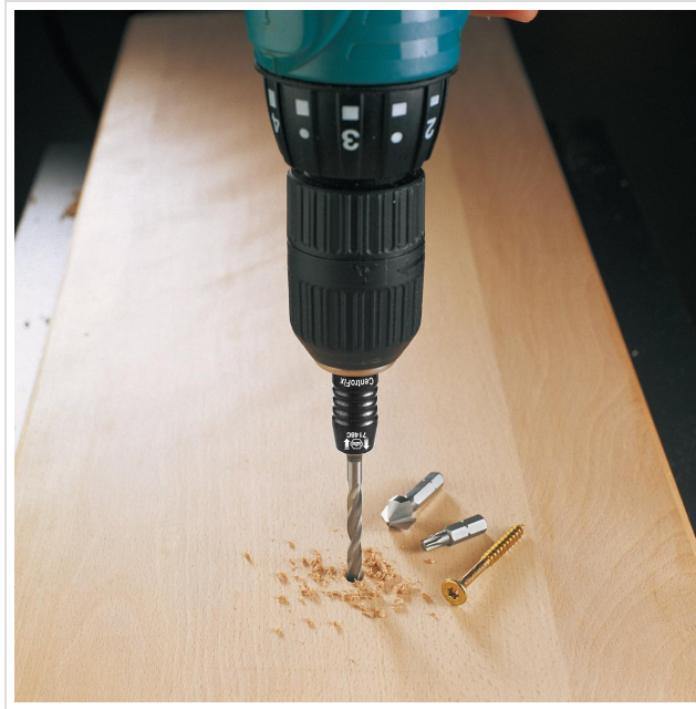
Image 4.2: The Wiha CentroFix holder attached to a power drill, holding a drill bit for precision work.
