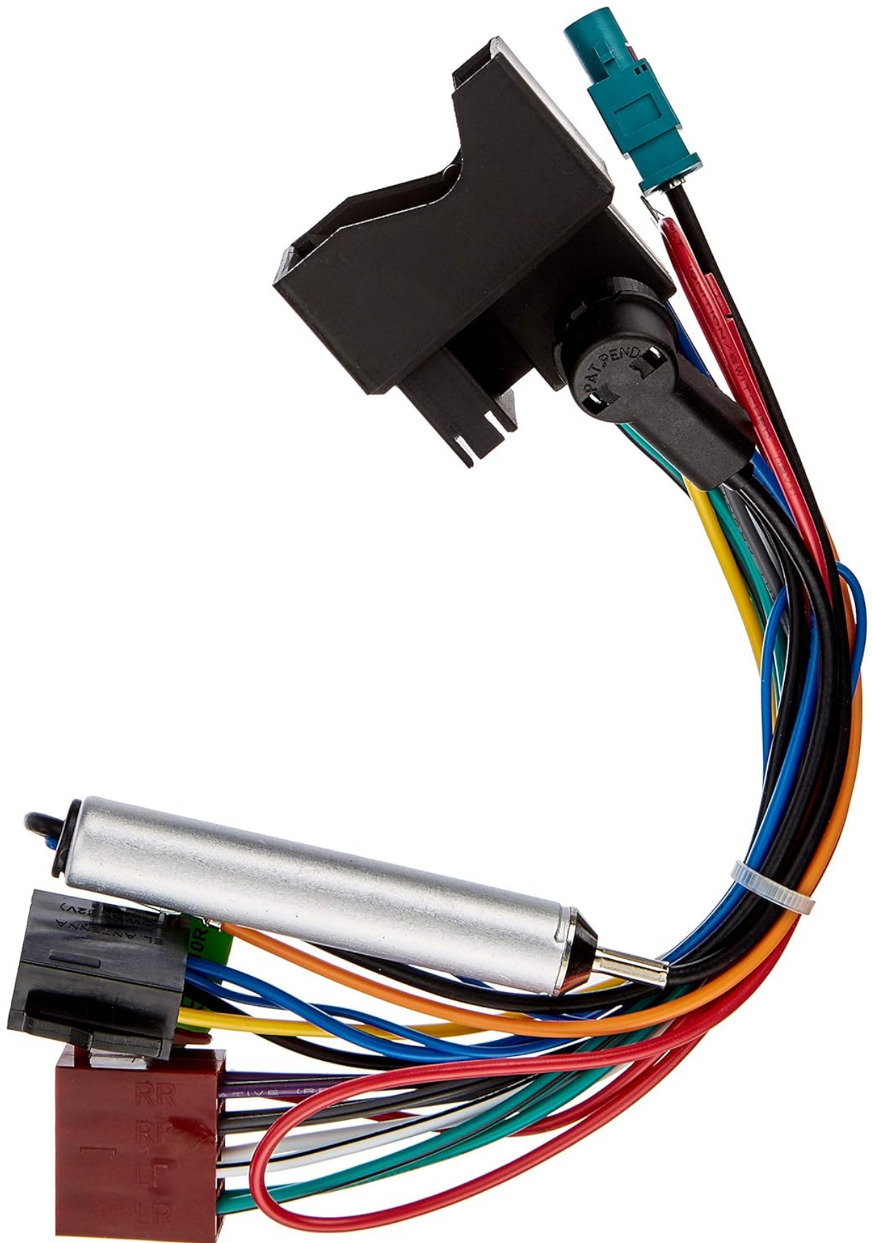
Figure 3: The ACV 1324-45 cable displaying both the vehicle-side Quadlock connector and the aftermarket radio's ISO connector, along with the antenna power line.
