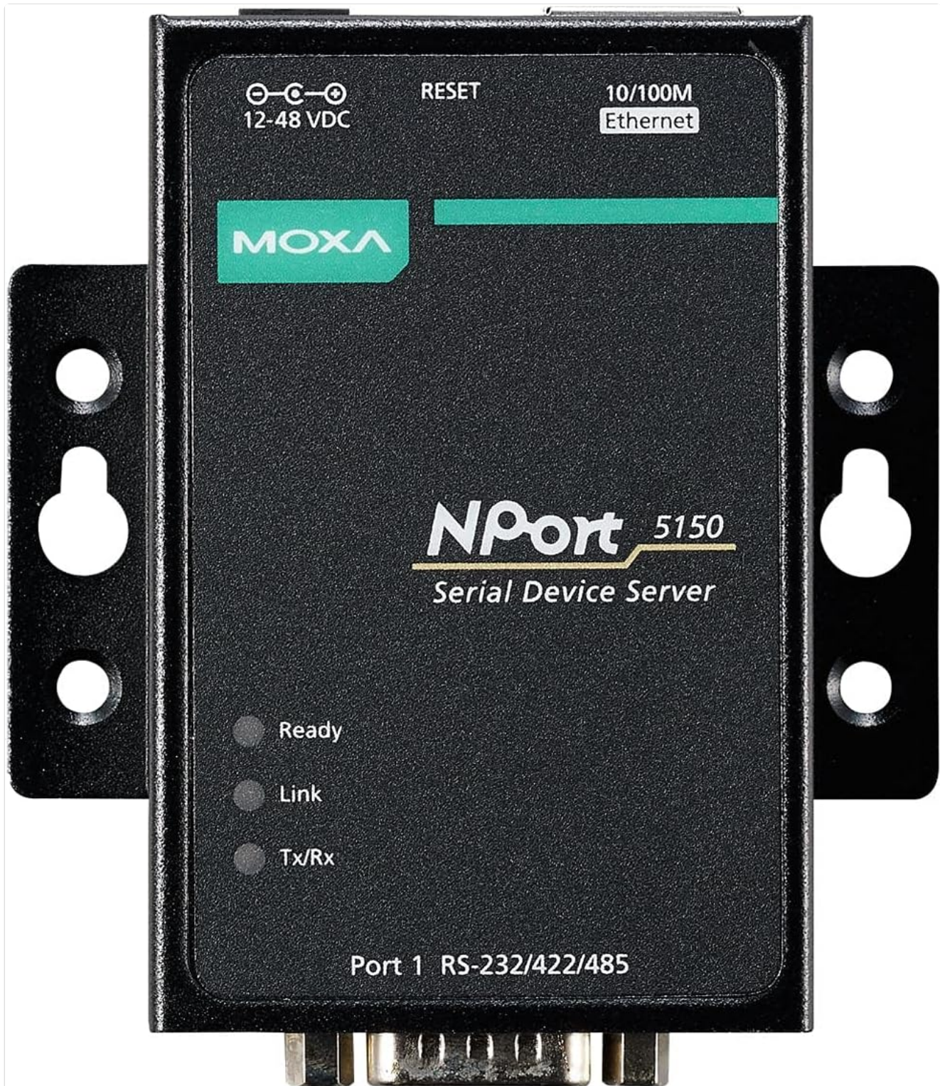
Figure 1: Front view of the MOXA NPort 5150 serial device server. This image displays the front of the MOXA NPort 5150 serial device server, highlighting its compact design and integrated mounting brackets. Visible features include the 12-48 VDC power input, RESET button, 10/100M Ethernet port, and the DB9 serial port labeled 'Port 1 RS-232/422/485'. LED indicators for Ready, Link, and Tx/Rx are also present.
