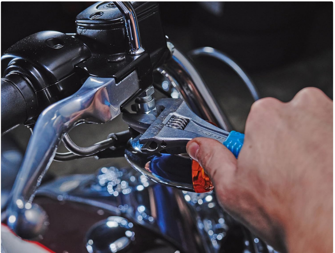
Figure 3: Illustration demonstrating the impressive 1.54-inch (39.12mm) jaw capacity of the WideAzz wrench.
