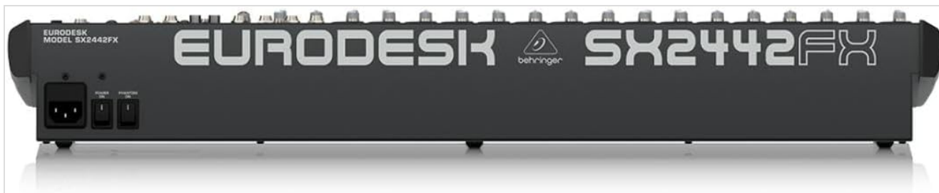
Figure 3.1: Rear panel of the SX2442FX, illustrating the power connection point.
