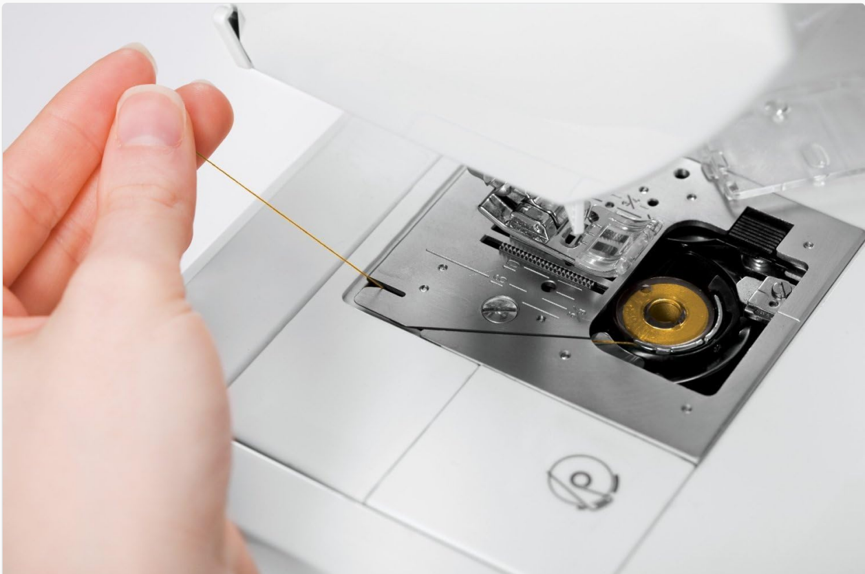
Image: Proper insertion of the bobbin into the bobbin case.
