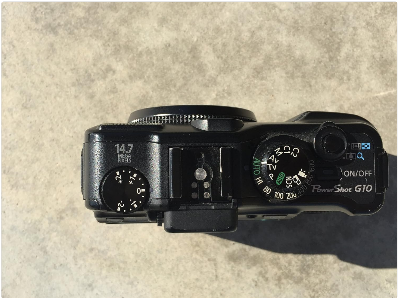
Image: Top view of the Canon PowerShot G10 camera, showing the mode dial, exposure compensation dial, and power button. This view highlights key controls for camera settings.
