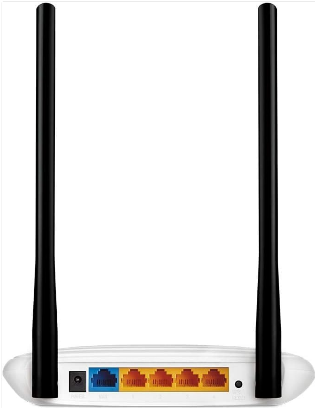
Figure 2: Rear panel of the TL-WR841N with power, WAN, and LAN ports.
