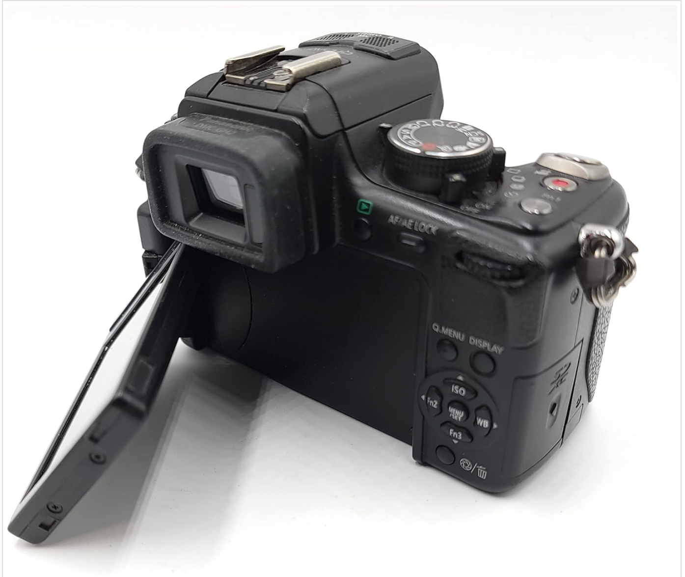
Figure 5.1: Rear view of the DMC-G1 with the LCD screen open, showing controls.
