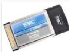
Figure 1.1: The SMC EZ Connect G Wireless Cardbus Adapter. This image shows the compact Cardbus adapter, designed to fit into a laptop's PC Card slot, with the SMC logo visible on its metallic casing.
