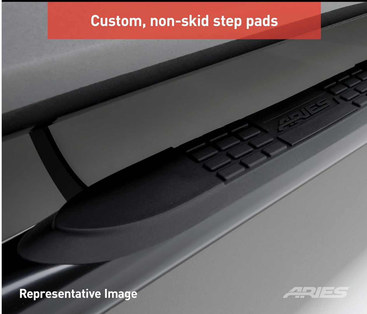
Image 2.2: Close-up of a non-skid step pad, illustrating its textured surface for enhanced grip.
