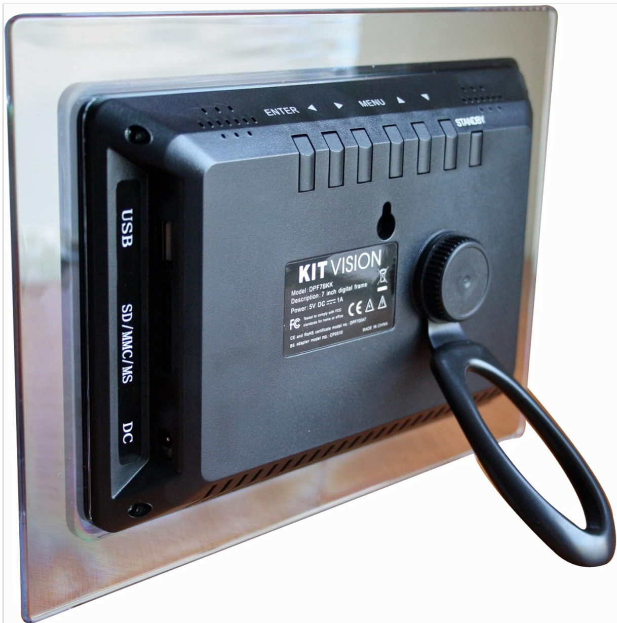
Figure 3: Rear view of the digital photo frame. Visible features include the USB port, SD/MMC/MS card slot, DC power input, control buttons (ENTER, arrows, MENU, STANDBY), and a detachable stand.
