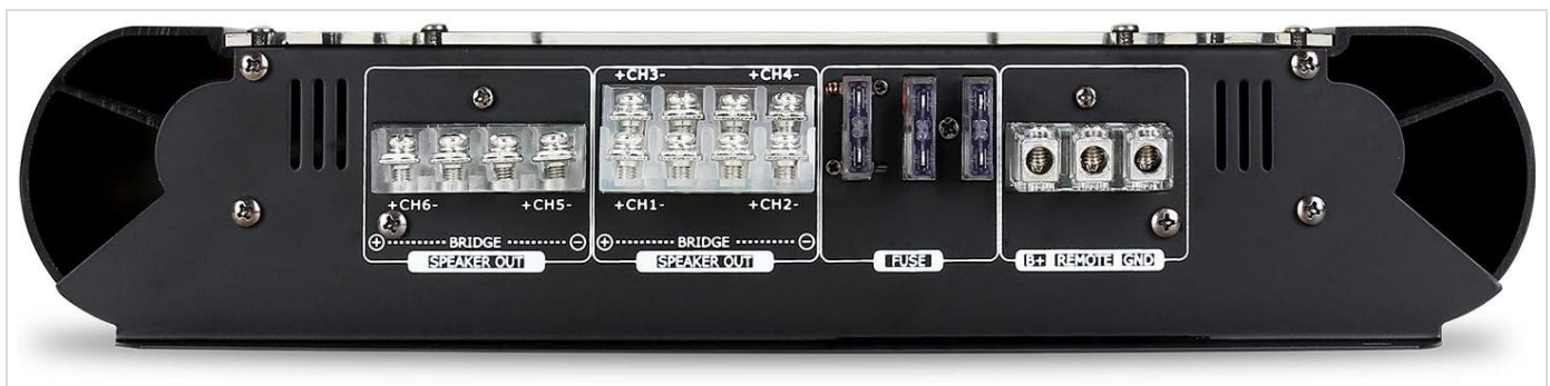
Figure 5.1: Rear panel of the amplifier, displaying the power input terminals (+BATT, REM, GND), fuse holders, and six speaker output terminals (CH1-CH6). The speaker terminals are clearly labeled for both positive and negative connections, with bridging options indicated.
