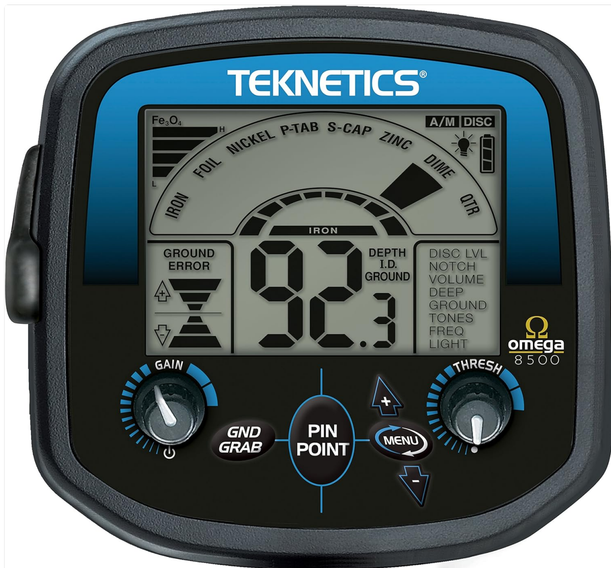
Figure 2.2: Close-up view of the Omega 8500 control panel, highlighting the LCD display, gain and threshold knobs, and pinpoint button.
