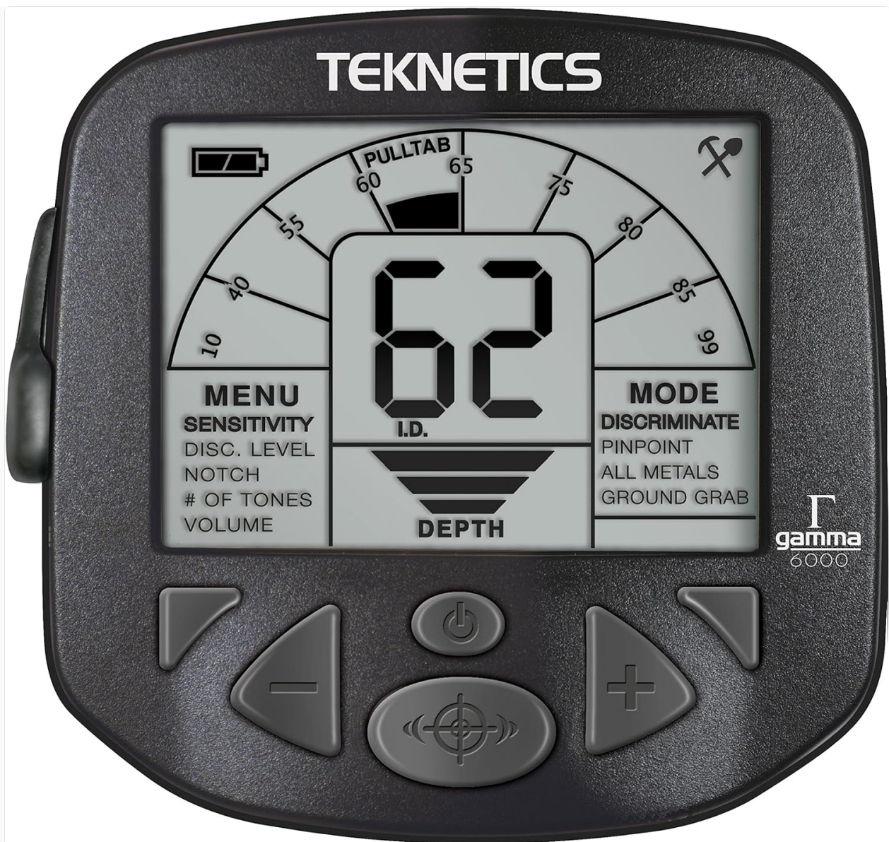
Image: A close-up view of the Teknetics Gamma 6000's LCD display and control buttons, showing menu options and target identification features.
