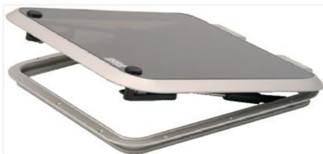
Figure 1: Bomar Low Profile Hatch 1000 Series, partially open. This image illustrates the anodized aluminum frame, the heavy-duty acrylic top, and the external hinge mechanism. The tie-down dogs are visible, securing the hatch in a slightly
