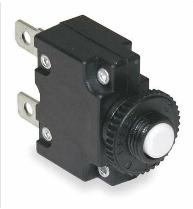
Figure 1: Carling Technologies Thermal Circuit Breaker. This image displays the compact black body of the circuit breaker, with two metal tab terminals extending from one side for electrical connections. On the front, a white push-button reset mechanism is visible, surrounded by a threaded collar for panel mounting.
