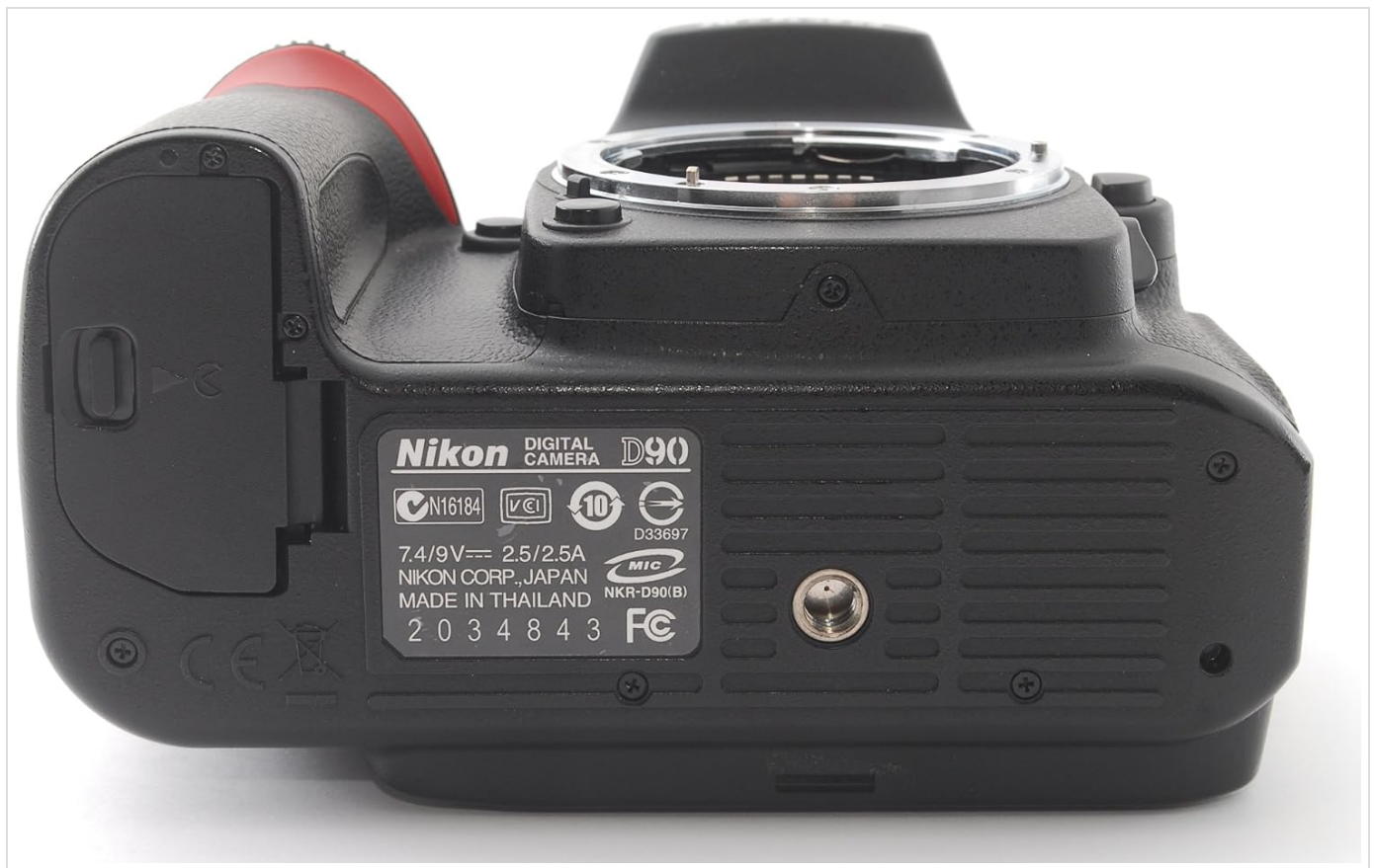
Figure 2: Bottom view of the camera, indicating the battery compartment.
