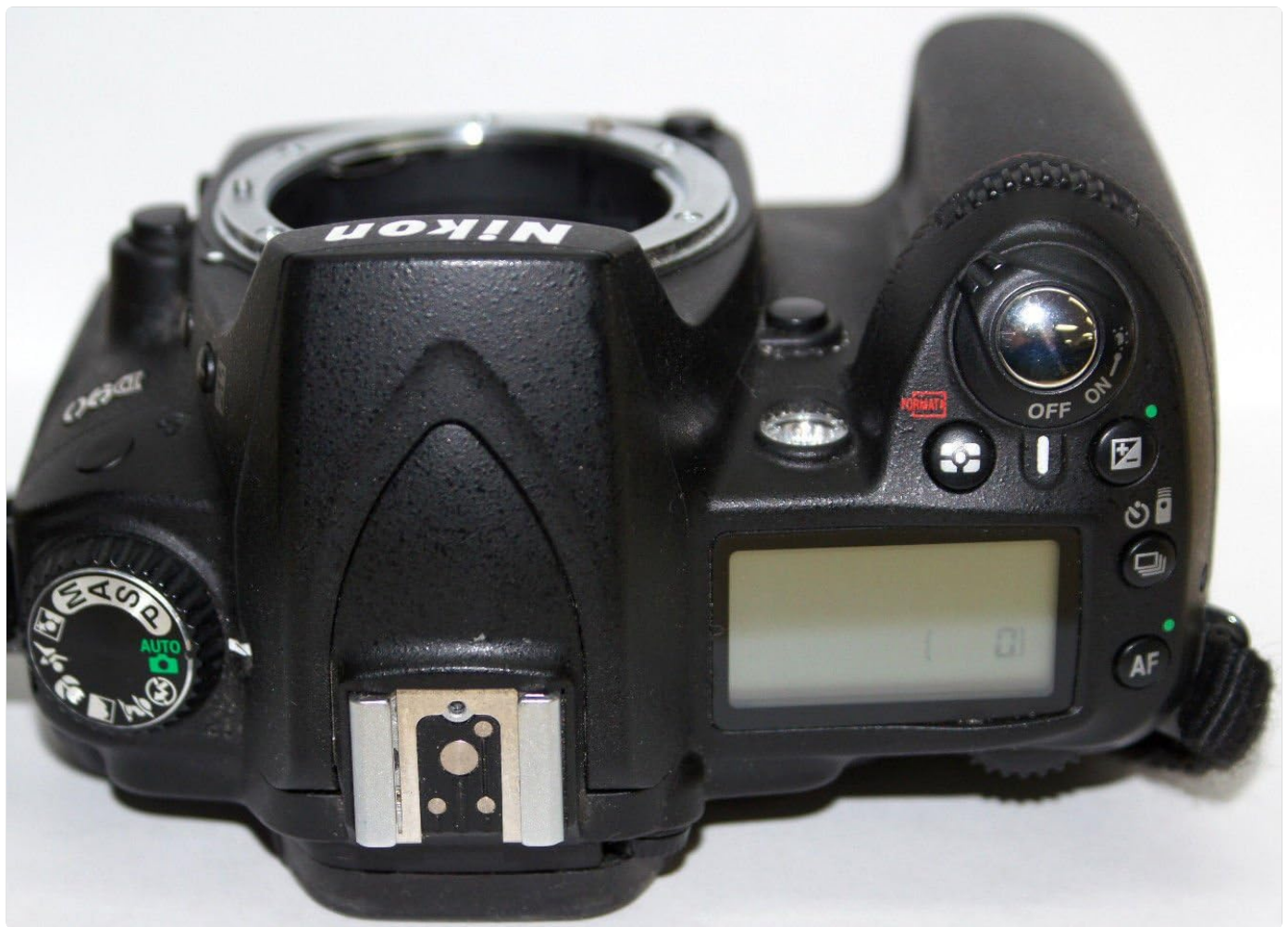
Figure 3.1: Top controls of the Nikon D90, including the power switch and mode dial.
