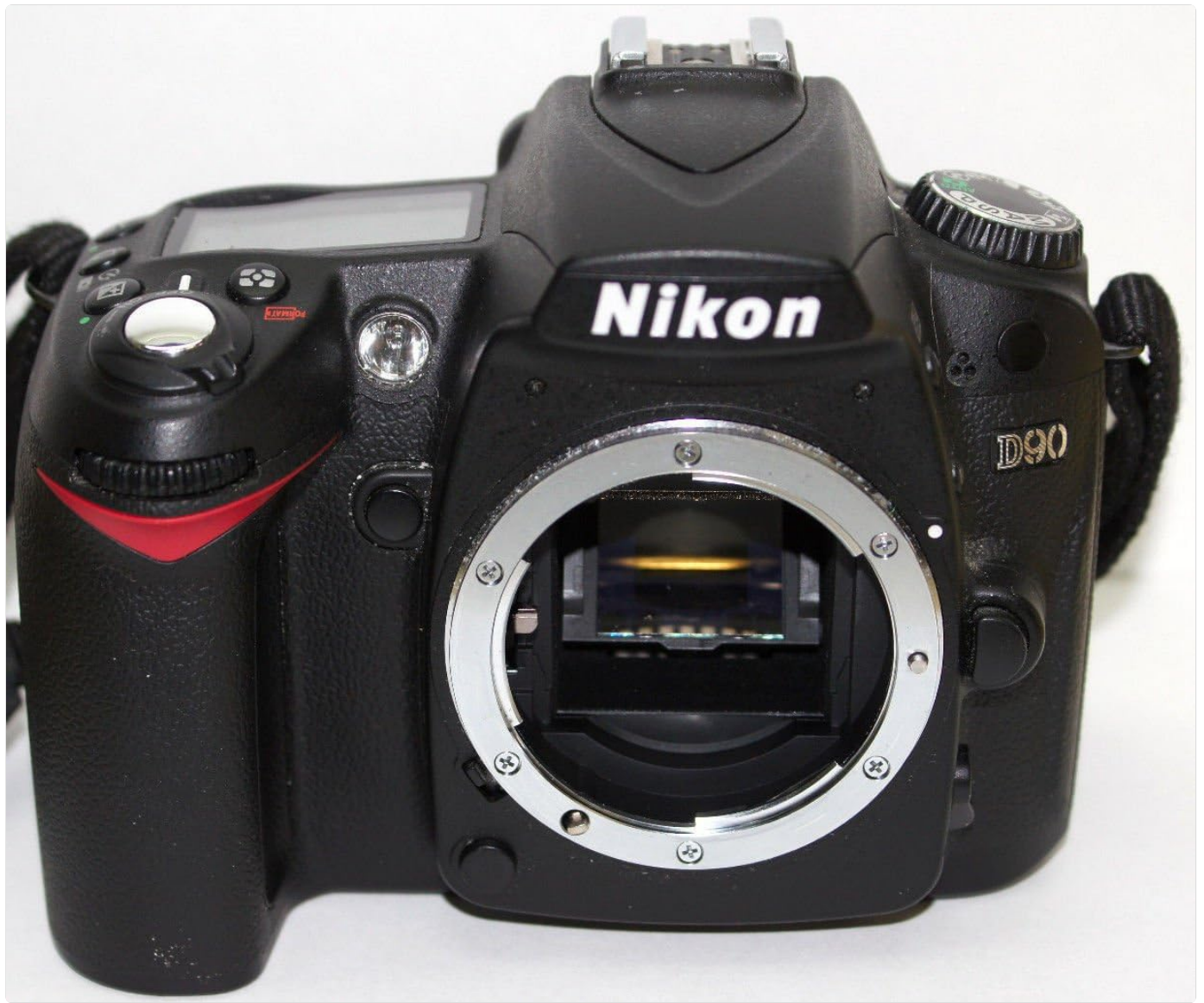
Figure 2.3: Front view of the Nikon D90 camera body, showing the lens mount.
