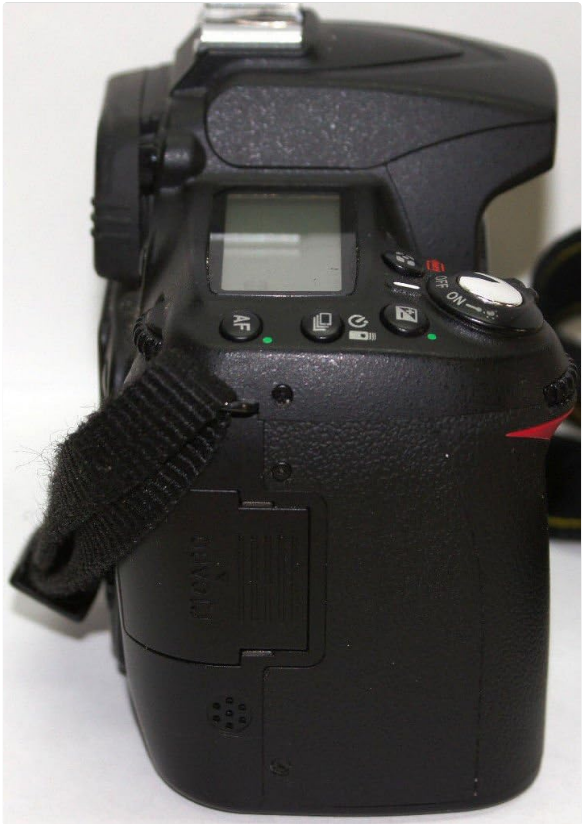
Figure 2.2: Location of the memory card slot on the Nikon D90.
