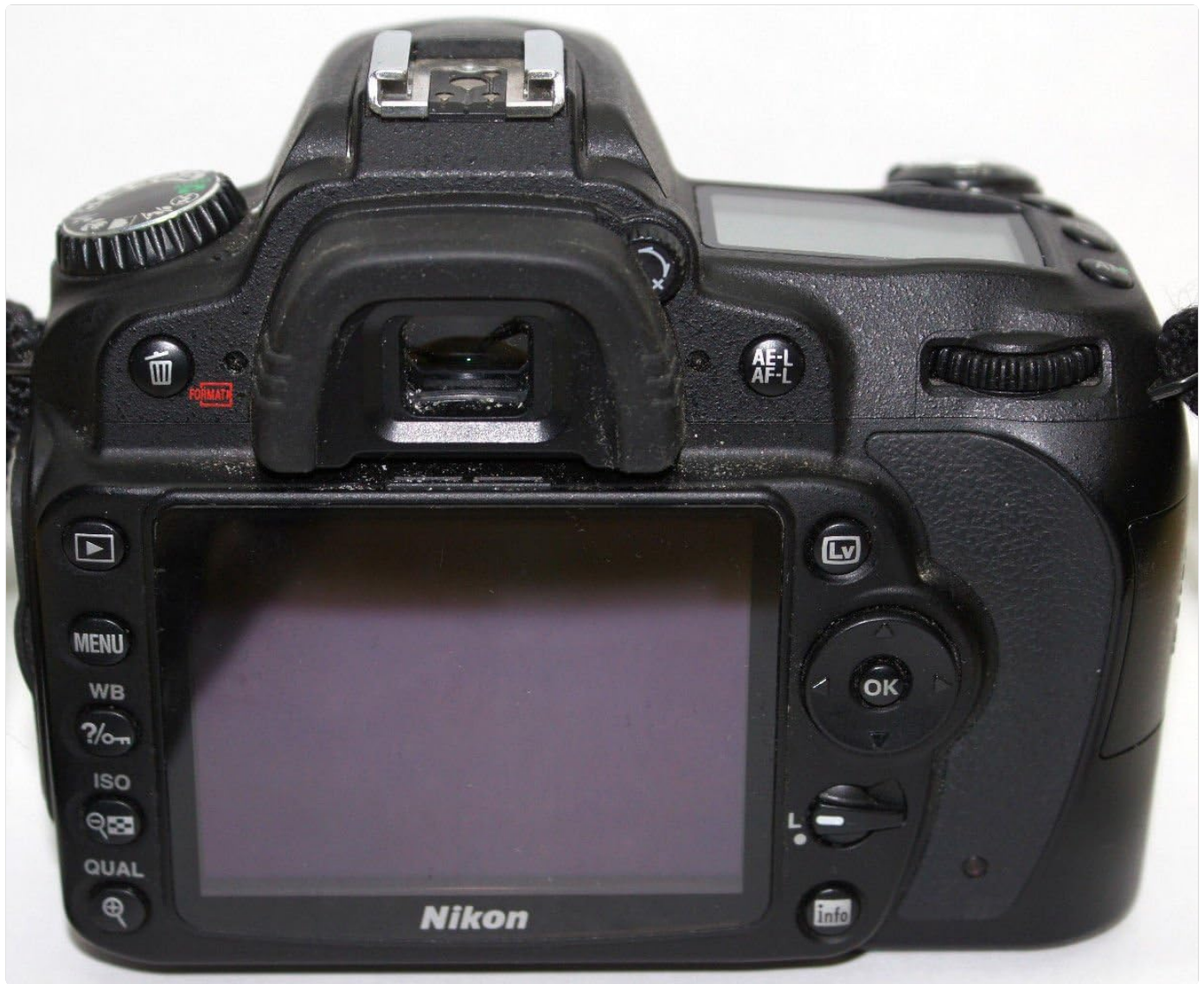
Figure 3.2: Rear panel of the Nikon D90, featuring the 3-inch LCD monitor and control buttons.
