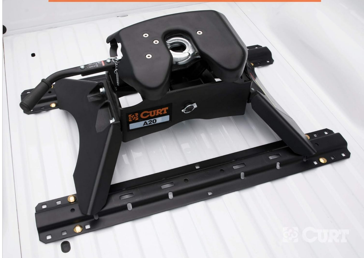
Image 4.1: A CURT A20 5th wheel hitch securely mounted on the installed 5th wheel rails in a truck bed. This demonstrates the final installed appearance.
