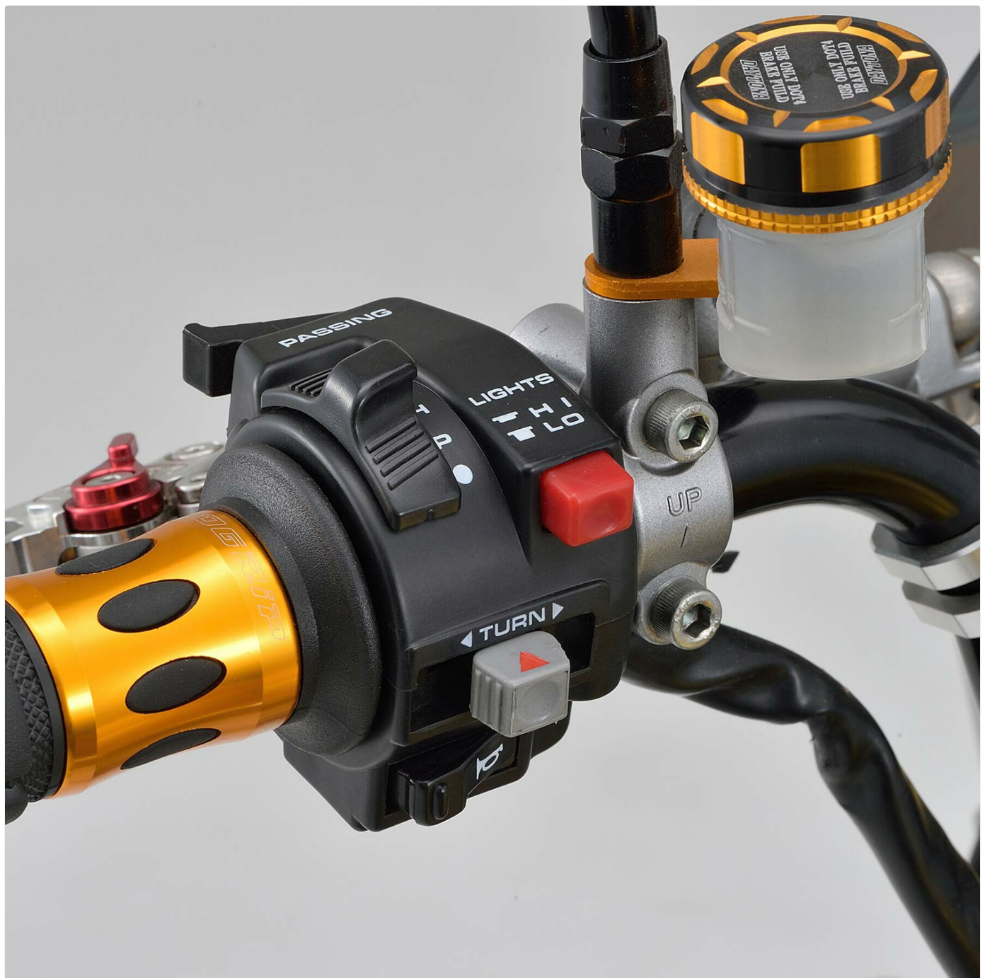
Figure 4: The Daytona 65602 switch mounted on a motorcycle handlebar, shown in context with other components such as the brake fluid reservoir and throttle grip. This view provides a practical perspective of the switch's placement and integration on a motorcycle.
