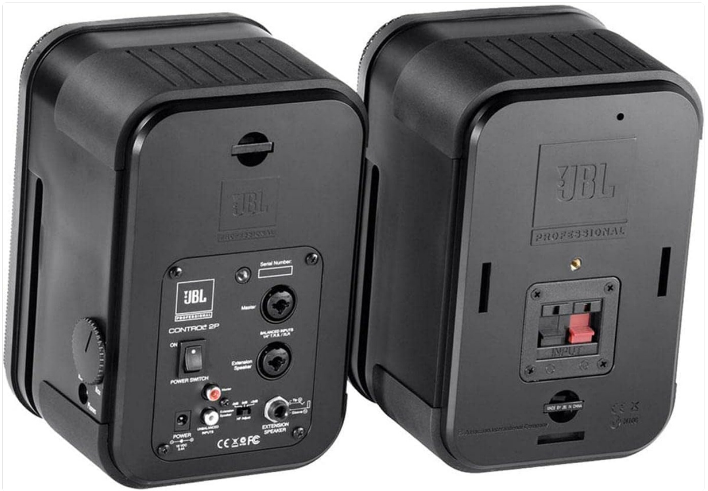
Figure 1: Rear panel of the JBL Control 2P Master Speaker, illustrating the balanced XLR, 1/4" TRS, and unbalanced RCA input options, along with the power connection and speaker output to the extension unit.
