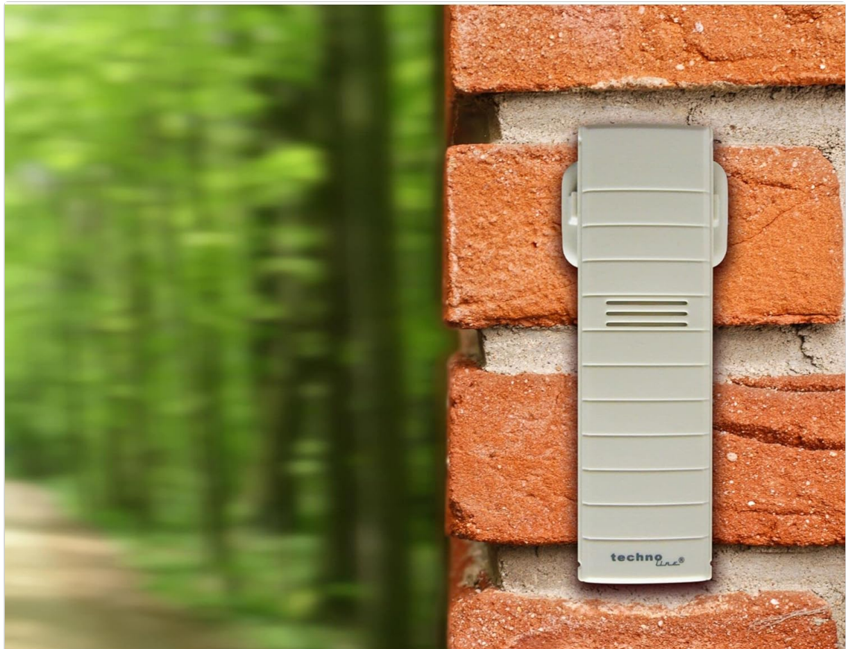
Figure 2: Recommended outdoor placement for the TX35-IT transmitter.
