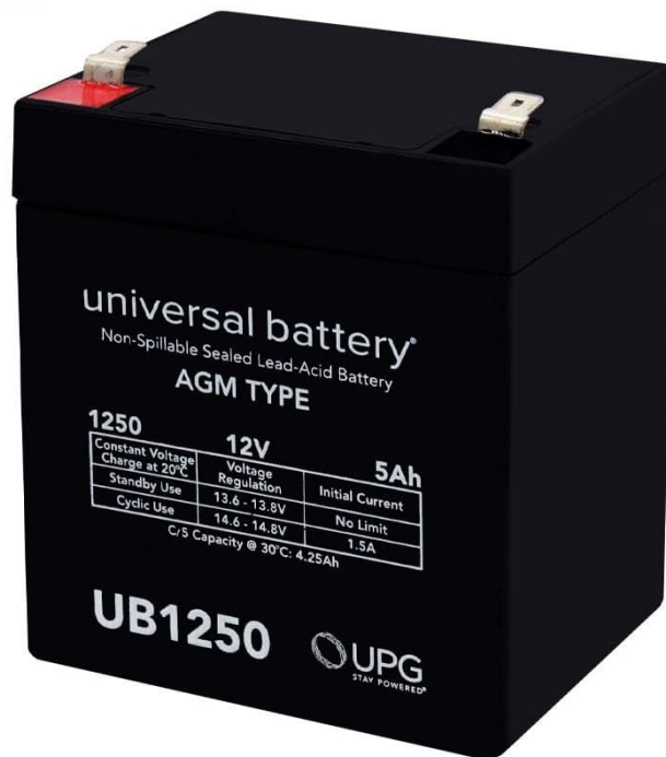
Image 2: Close-up of the UPG UB1250 battery label, detailing constant voltage charge at 20°C for standby use (13.6-13.8V) and cyclic use (14.6-14.8V), with initial current less than 1.5A.
