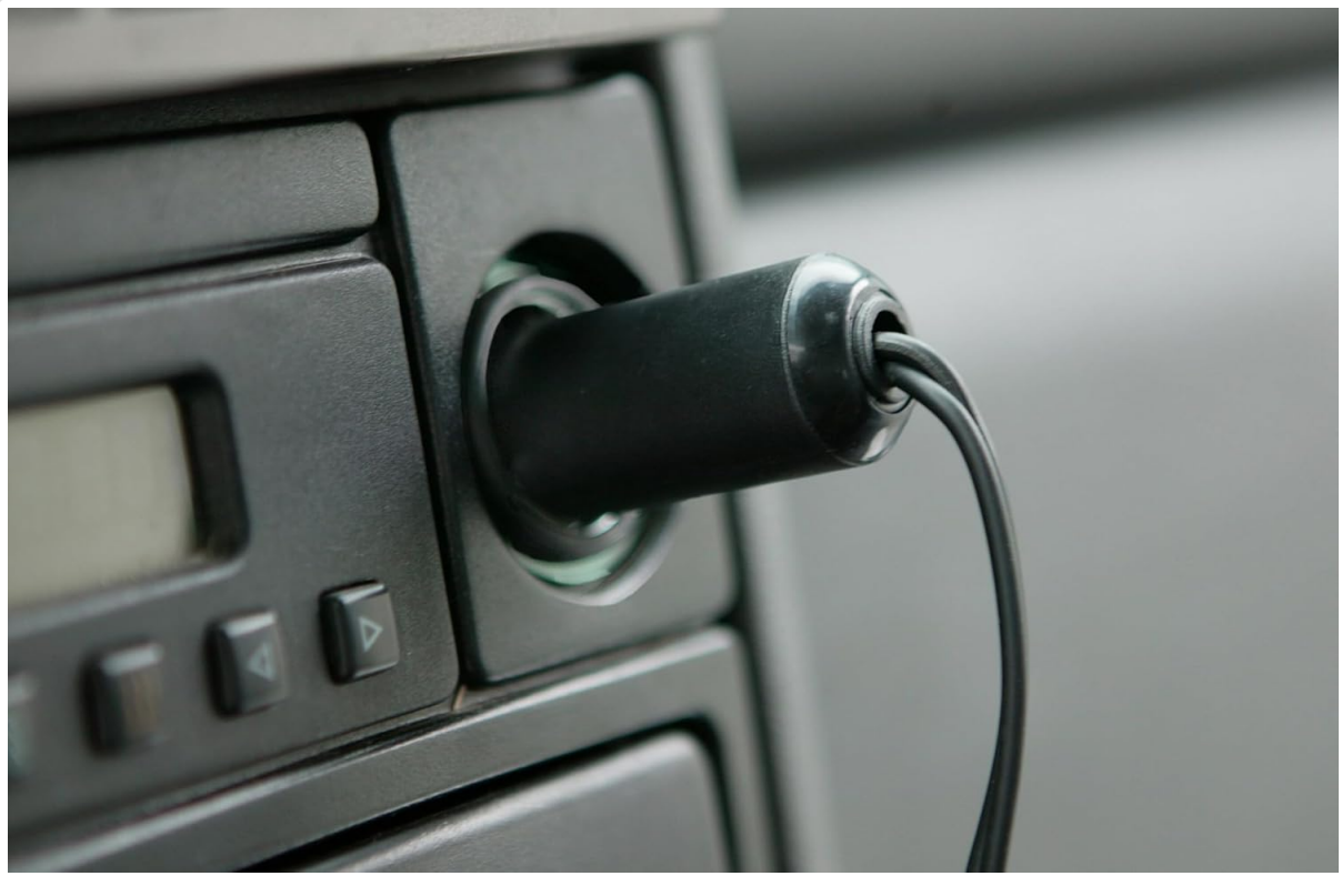
Figure 4: Connecting the 12V power plug to the car socket.
