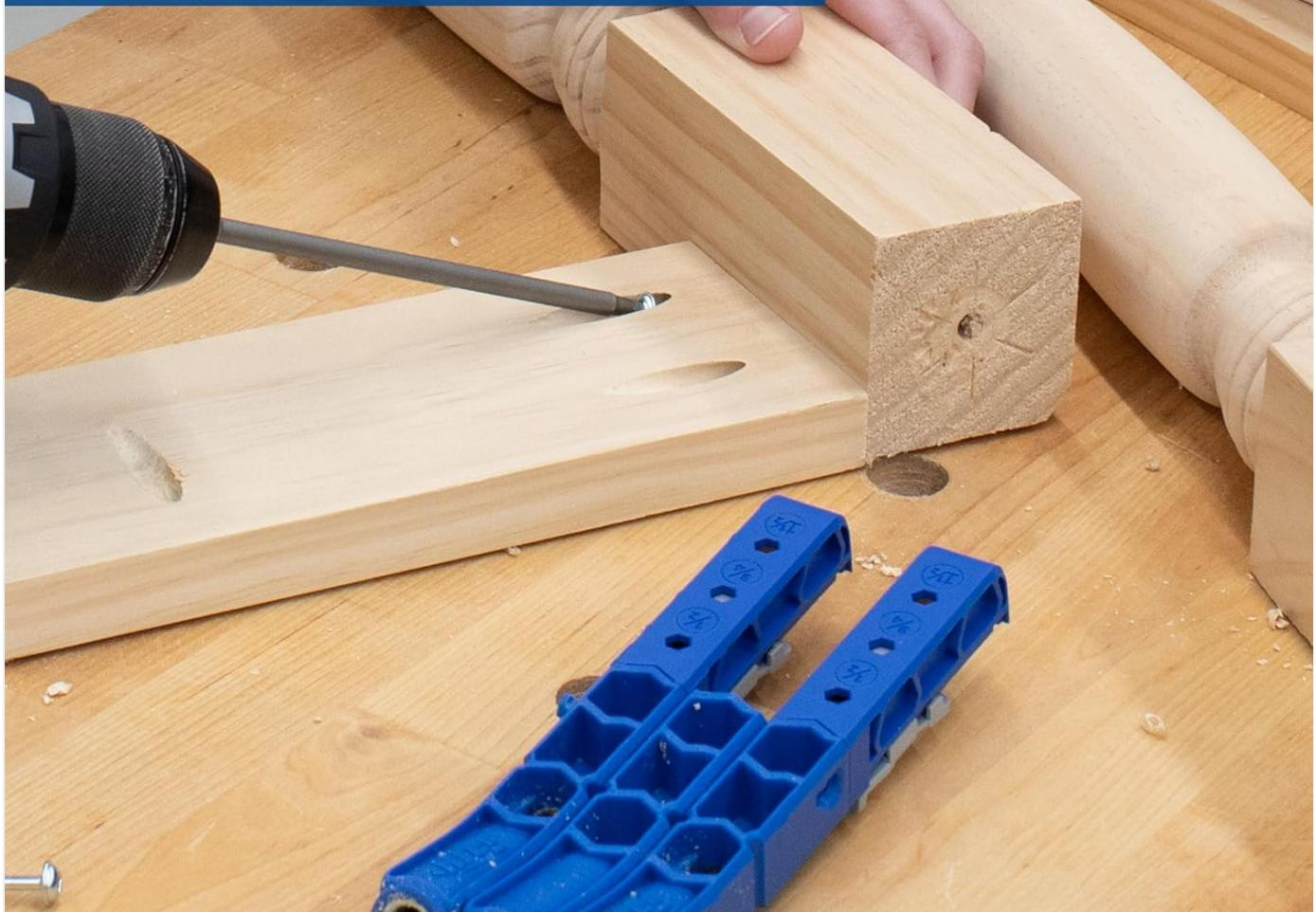
The image illustrates the process of drilling pocket holes, a preparatory step before driving the screws.
