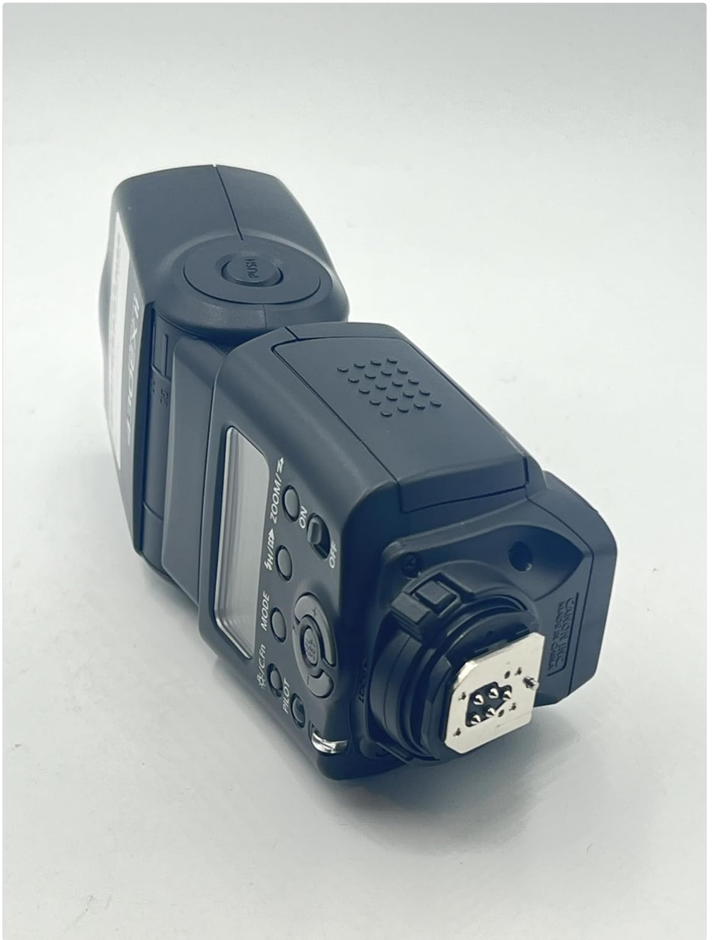
Figure 3: Bottom view of the Speedlite 430EX II, highlighting the hot shoe mount for camera attachment.
