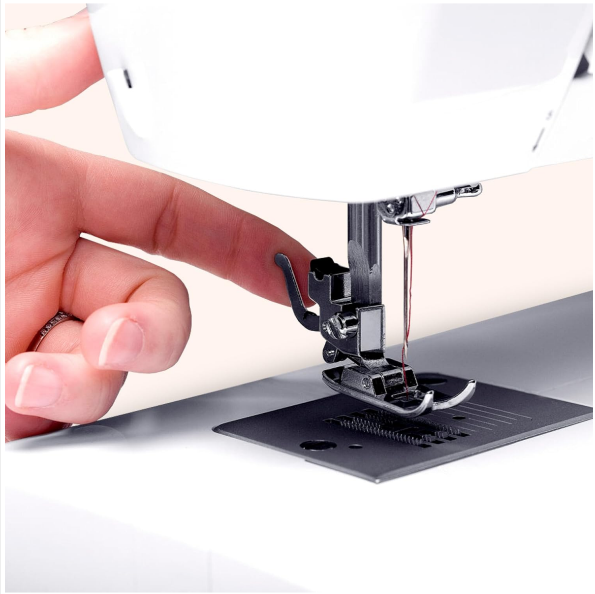
Image: A close-up of the buttonhole presser foot, designed for creating uniform buttonholes.
