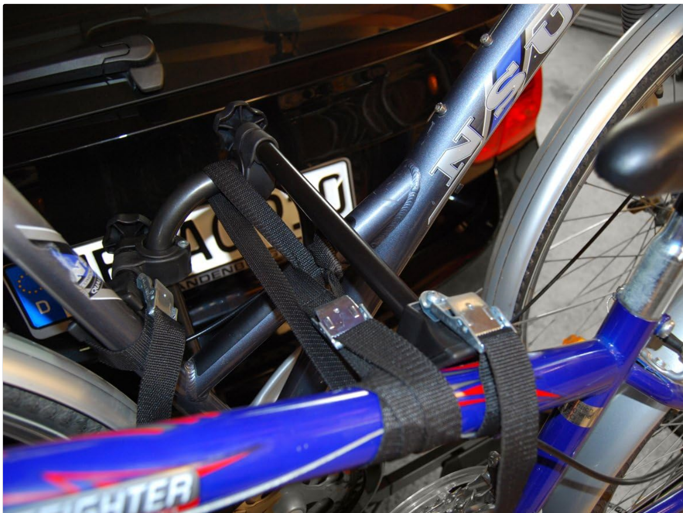
Image 1.1: The Eufab 11231 Long Frame Holder in use, securing a bicycle frame to a carrier.
