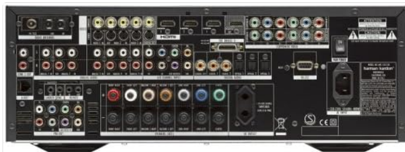
Figure 2: Rear panel of the Harman Kardon AVR 355, showing various audio, video, and speaker terminals.
