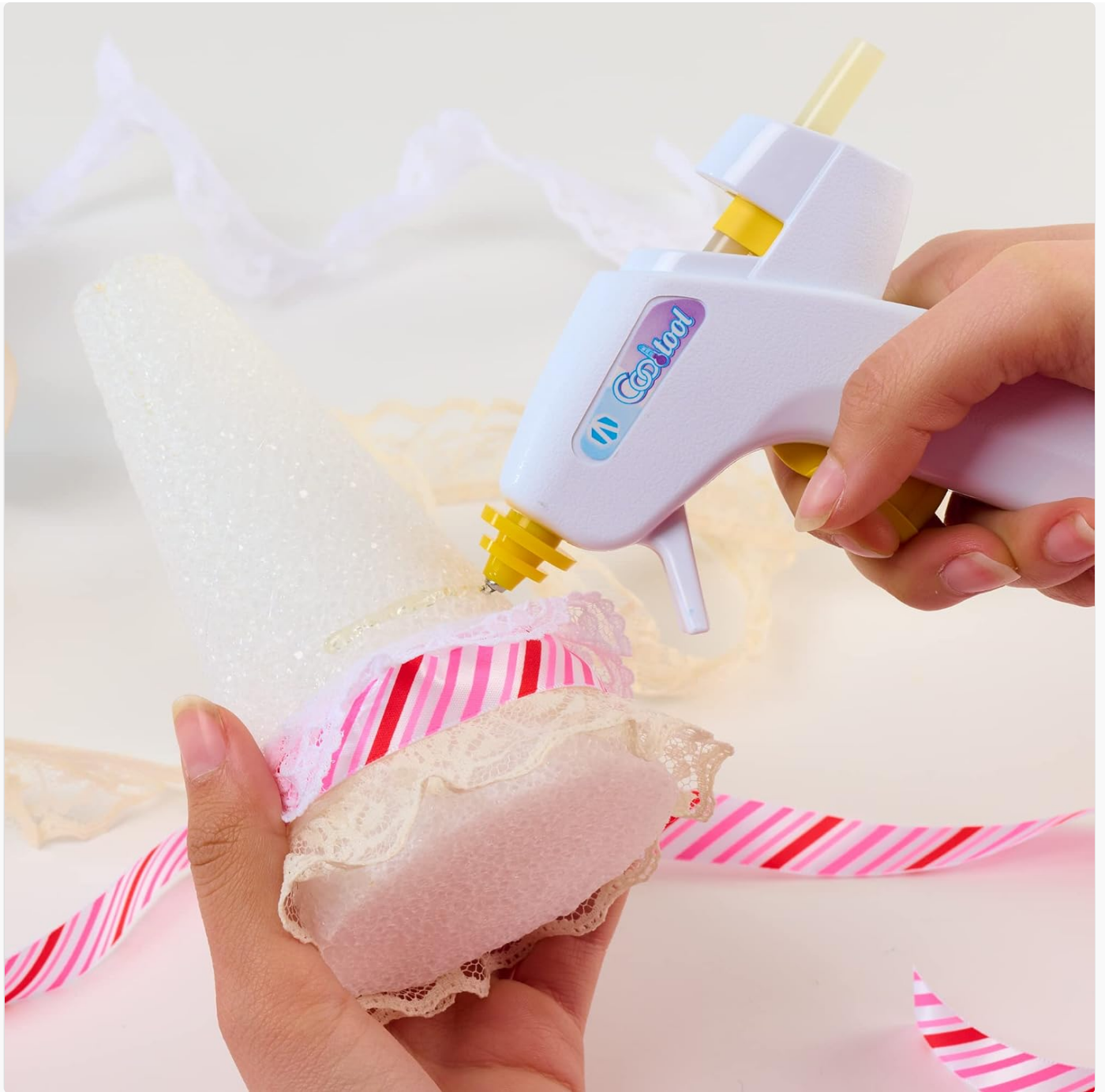
Image 4.2: A person applying glue with a mini glue gun to attach a decorative ribbon to a white craft cone, showcasing its use for delicate assembly.
