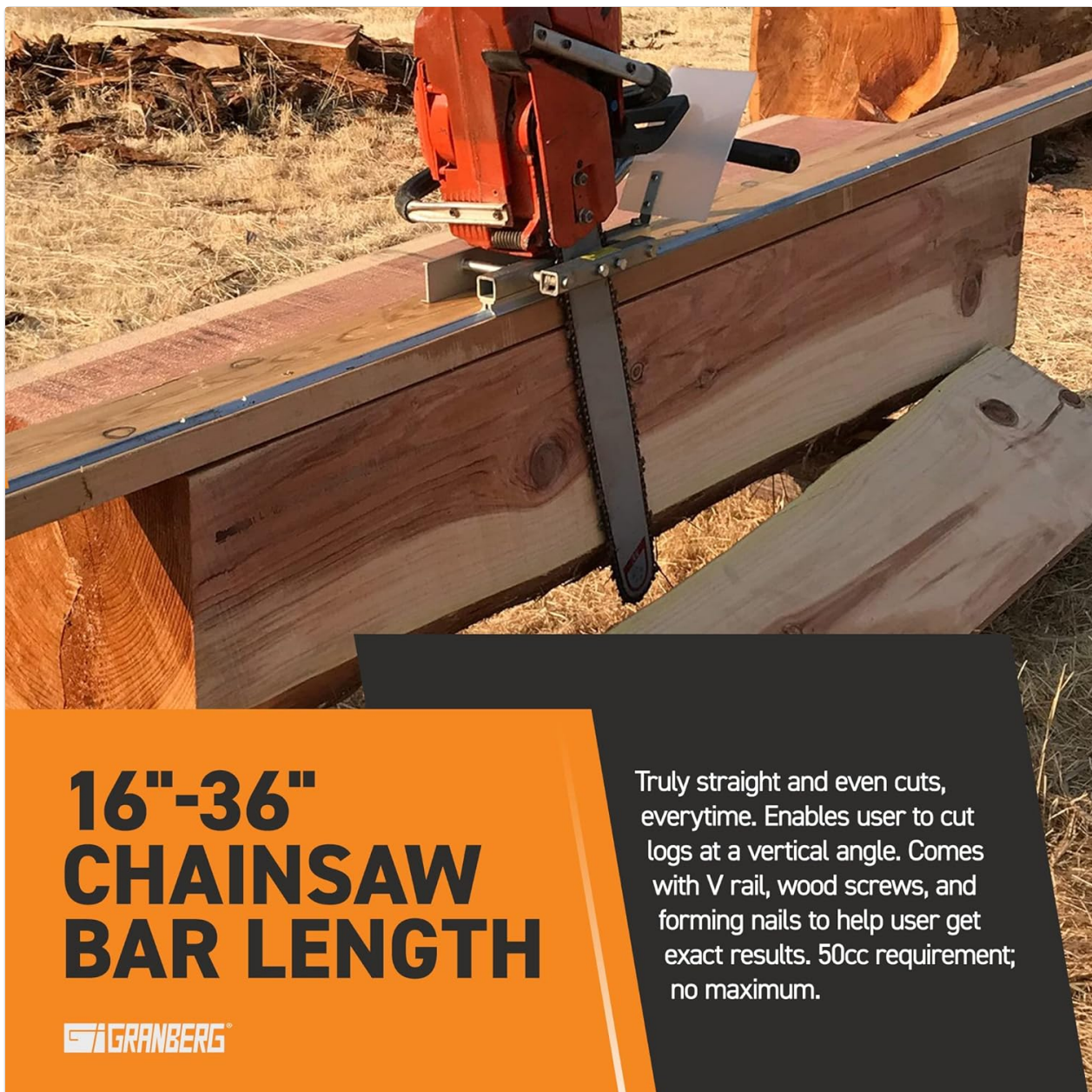
Image 3: The G555B Edging Mill supports chainsaw bar lengths from 16 to 36 inches.
