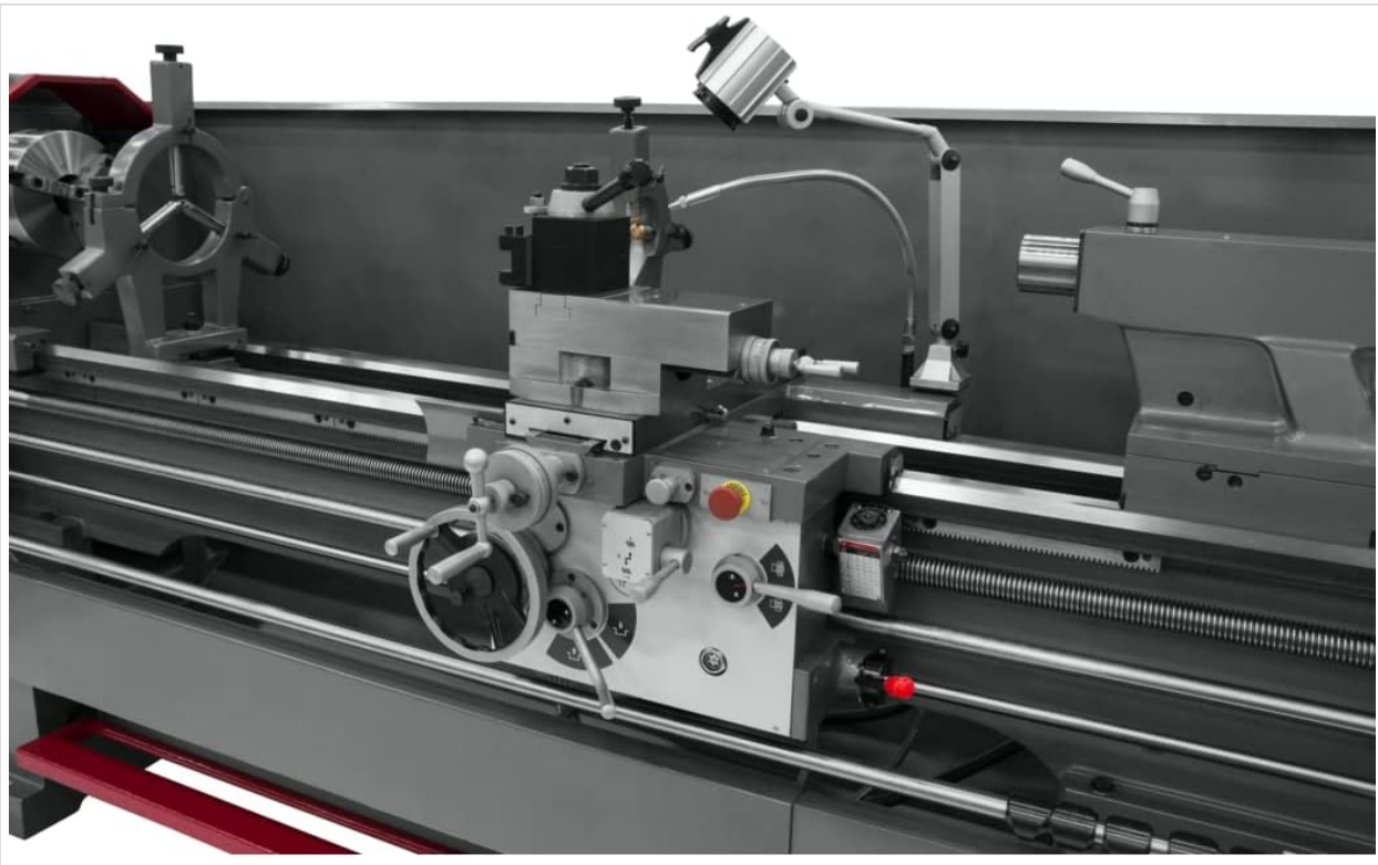
Figure 5: Detailed view of the carriage, tool post, and lead screw.
