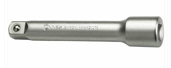
Image: A silver-colored Connex COXT570125 extension bar made of chrome-vanadium steel. It features a 1/2-inch square drive on one end with a ball detent for securing sockets, and a 1/2-inch square female drive on the other end for connecting to a ratchet or other drive tool. The Connex logo and 'CHROM VANADIUM' are embossed on the shaft.
