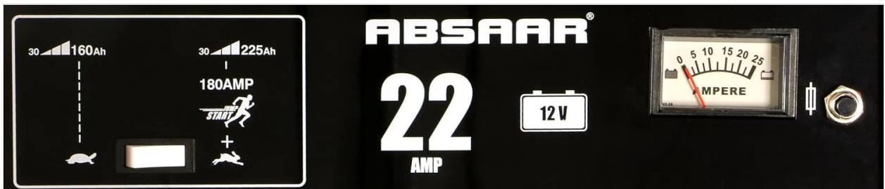
Figure 3.2: Close-up view of the charger's front control panel. It features a switch for charging modes (standard/fast), an ampere meter, and indicators for battery capacity ranges.
