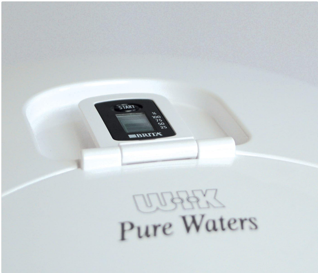
Figure 3: The digital display on the kettle lid, which indicates the remaining filter life and prompts for filter replacement.
